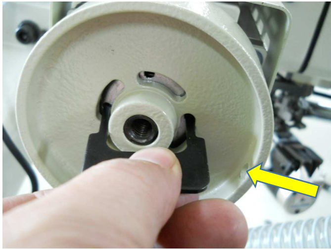
Position of needle bar height adjust here Special tool is included in the motor.
