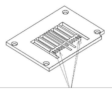
The black marks in the needle plate show factory needles set up
