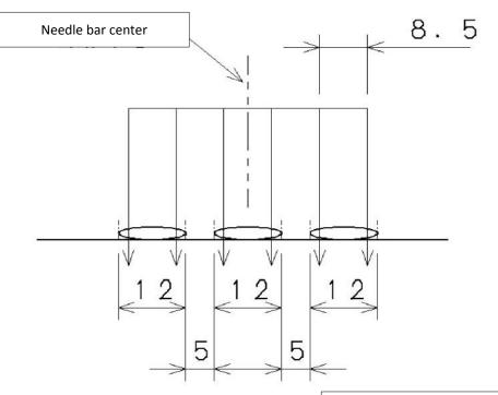
Measurements are in mm
