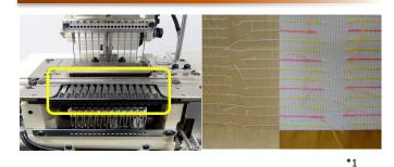
Increase in productivity up to <u>160%</u> Reducing working hours of operators Less thread wastage (Save approx.10cm per needle) Saving labor cost No helper needed for trimming thread Reducing the troubles Automatic needle positioning
