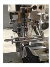
Design of the smocking can be easily changed from backside of the machine by changing the cam, changing thread variation
