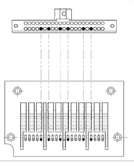
The black marks in the needle plate show factory needles set up
