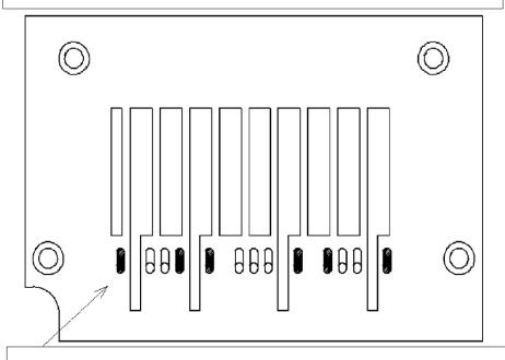
The black marks in the needle plate show factory needles set up
