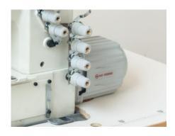
**Direct drive motor**Powerful running and high efficiency!
