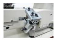
• Turn down bracket For attaching folder for waistbanding operation.
