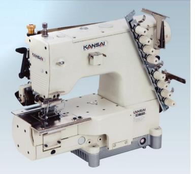
FBX series is a cylinder bed, 2-6 needle double chain stitch machine with needle feed. It is designed for sewing waistbands of medium heavy to heavy material such as jeans and working pants. As needle feed and lower feed are linked, both feeding amounts can be adjusted at the same time by push button operation. An additional rear puller is available as option.
