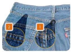
Solutions for uneven stitches at cross section upper puller, synchronized with feed dogs, gives most efficient feeding for thicker material
