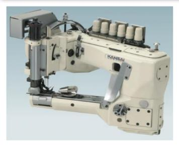
3 needle, double chain stitch, feed-off the arm machine, with a puller and differential feeding system \*\*Lapseam folder is included\*\*
