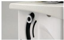
Lever type adjustment enables to make partial shirring.
