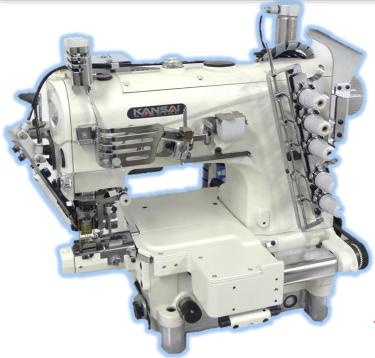
3 needles, super ultra small cylinder bed, Top and bottom cover stitch machine (with automatic thread cutter)
