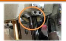
Needle bar oil return system Protects the fabric from the oil stain
