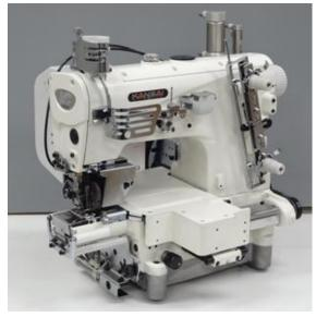
Exclusive puller feeding with differential feed dog mechanism
