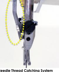
**Needle Thread Catching System** (only for SPX211) Prevents skip stitches by securing the need thread feeding
