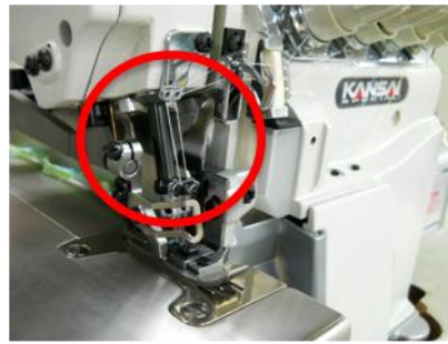
Diamond Like Carbon(DLC) coated needle bar and upper looper holder Ensure durability and reliability and help machines run in high speed
