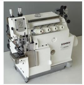
2 needles 4 threads overlock with 148mm circumference cylinder with top feed mechanism.
