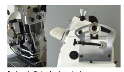
**Equipped with top-feed mechanism** Top feed front- back: 1-6mm Top feed up-down: 4.5mm
