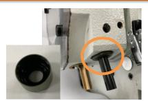
Needle bar oil seal is applied
