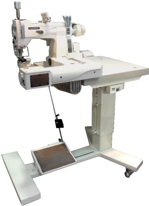
3 needle, feed-off the arm, double chain stitch for heavy duty material with differential feeding mechanism
