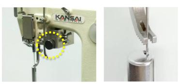
Upper Feed System Equipped with a dial knob, micro adjustment is possible for feed amount.
