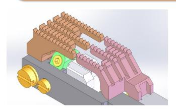
Differential feed mechanism ensures prevents puckering
