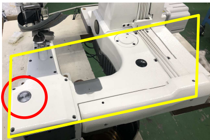
Push button stitch length adjustment
