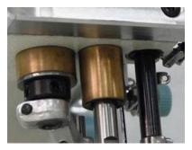
Double layered oil seal is applied in the needle bar and the presser foot. This new oil seals protect your garment from oil stains.
