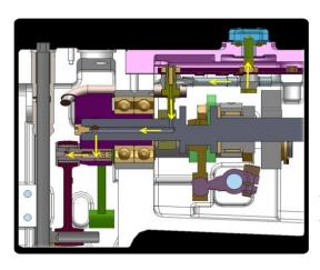
State of the art lubrication mechanism circulates the oil to the needle bar link bearing. This mechanism reduces noise and vibration.
