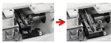
Sliding thread take-up mechanism By pulling the lever, the looper thread take-up slides down toward the operator. This mechanism makes easy to thread and troubleshoot.
