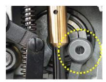
Needle bar stroke can be changed with only a screwdriver. 31mm ⇔ 33mm
