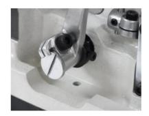
Micro adjustable looper holder With this new looper holder system, gauge adjustment become much easier.
