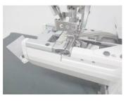
NR9803GP-UTA model includes the pneumatic thread trimmer and presser foot lifter
