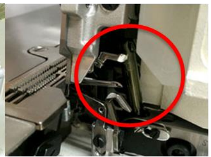
Diamond Like Carbon(DLC) coated needle bar and upper looper holder Ensure durability and reliability and help machines run in high speed
