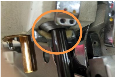
Needle bar oil return system Protects the fabric from the oil stain
