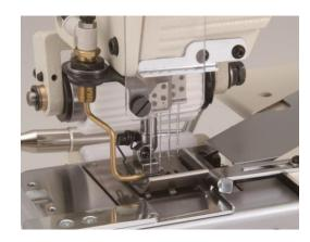
Suitable for attaching elastic operation with double flatlock seam on men's underwear
