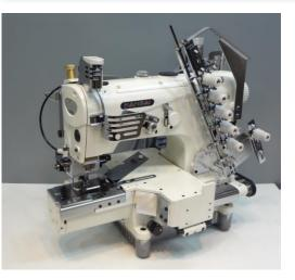
4 needle, cylinder bed, double chain stitch machine for attaching elastic
