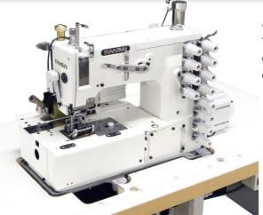
6 needle flat bed, double chain stitch machine for denim waistband attaching. The machine equipped with a fabric cutter, skip stitch device and foot lifter
