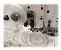
The machine has 2 spreaders and each spreader has 3thread eyelets. Design can be changed by variation of threads combination.
