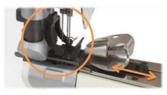
1. Solutions for uneven stitches at cross section upper puller, synchronized with feed dogs, gives most efficient feeding for thicker material
