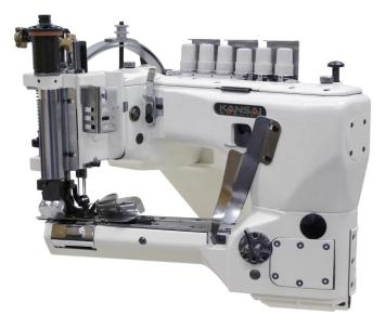
3 needle, feed-off-the-arm double chain stitch machine for lap seaming.
