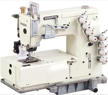
DFB series are flatbed, multi-needle double chain stitch machines. This series is multi-purpose such as attaching elastic, attaching waistband,
