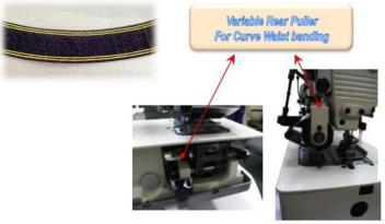
Flat-Bed double chain stitch machine for CURVED waist banding with preinstalled Japan made 15 needle gauge and turn down folder bracket.
