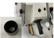
Needle bar oil seal is applied This mechanism protects the fabric from the oil stain
