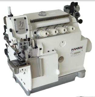
2 needles 4 threads overlock with 148mm circumference cylinder with top feed mechanism.
