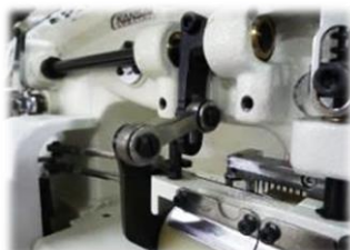
Can easily adjustment the puller feed by outside
