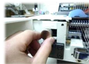
Dial feed amount adjustment and we can change shirring condition while sewing by dial
