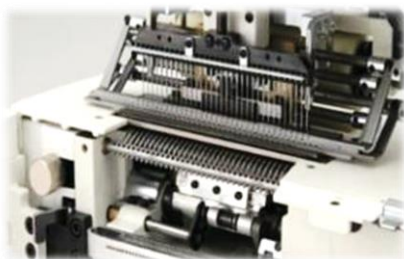
4 spreaders for the decorative thread increase the number of design patterns.
