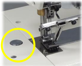
Adjusting stitch length With the push button
