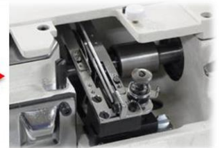
Slide type thread take-up base makes threading and troubleshooting easier
