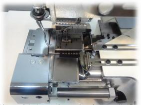
It is possible to use 2 needle of coverstitch and 3 needle of chain stitch in one operation. Best-suited for sports wear and trunks pants.
