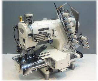
2 needle for bottom cover stitch and 3 needle for double chain stich for attaching elastic.
