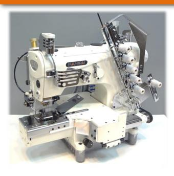
4 needle double chain stitch machine with horizontal looper movement mechanism. It can be used for attaching endless or pre-closed elastic. Major feature of this series is the cylinder bed. This feature gives you benefits when you work with trunks, boxers, and similar garments.
