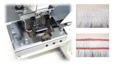
Making 2 line of flat lock stitch in one operation
