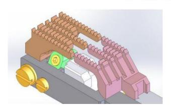
Differential feed mechanism ensures prevents puckering
