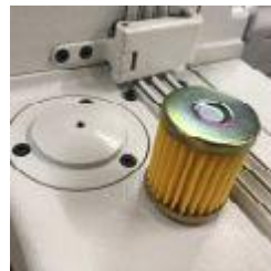
Full automatic lubrication with Oil filter
