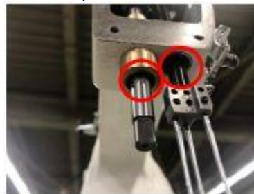
DLC coated Needle bar and oil seal achieve high
