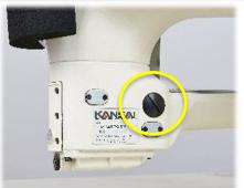
Differential feeding movement can be changed from 1:1.5 to 1:0.5 with
