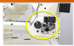
Stitch length & differential ratio can be adjusted by levers from out side of the machine.
