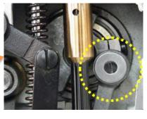
Needle bar stroke can be changed with only a screwdriver. 31mm ⇔ 33mm
