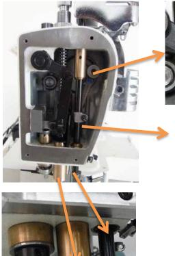
Double layered oil seal is applied in the needle bar and the presser foot. This new oil seals protect your garment from oil stains.
