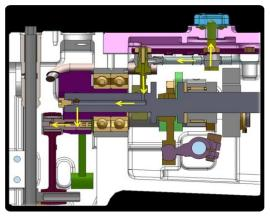
State of the art Lubrication mechanism circulates the oil to the needle bar link bearing. This mechanism can reduce noise and vibration. Above picture shows the flow of the oil while machine running.
