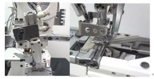
Pneumatic presser foot lifter and thread cutter reduces the operator's stress and helps increasing in productivity
