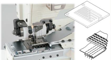
Without bottom cover stitch, for attaching pre-closed elastic tape with 4 needle, 4 loopers and 8threads.
