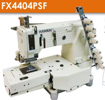
FX4404PSF are **Cylinder-bed**, multineedle double chain stitch machines with smooth puller for shirt fronting.
