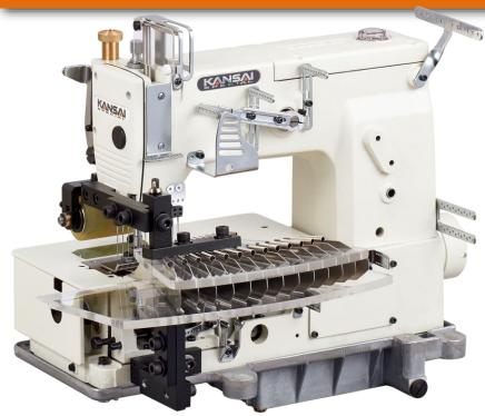
12 needle, flatbed, double chain stitch machine for pintucking operation.
