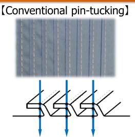
\* the needle is pierced into three pieces of fabric, the fabric is fixed and is often used for sewing decorations
