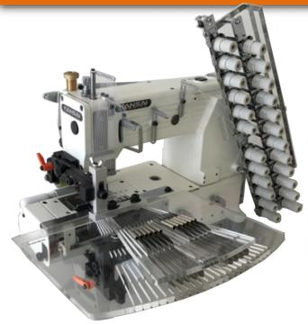
10 needle, cylinder bed, double chain stitch machine for pintucking operation. Perfect for the guayabera(Cuban shirt).
