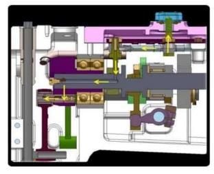
State of the art lubrication mechanism circulates the oil to the needle bar link bearing. This mechanism reduces noise and vibration. Left picture shows the flow of the oil while machine running.
