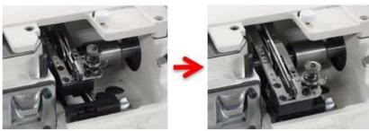
Sliding thread take-up mechanism By pulling the lever, the looper thread take-up slides down toward the operator. This mechanism makes easy to thread and troubleshoot.
