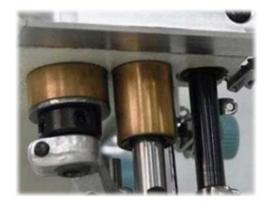
Double layered oil seales applied in the needle bar and the presser foot. This new oil seals protect your garment from oil stains.
