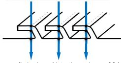
\* the needle is pierced into three pieces of fabric, the fabric is fixed and is often used for sewing decorations
