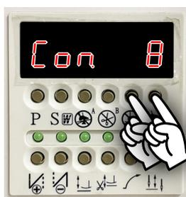
Set the number of condensation stitches and press[S] to conform.
